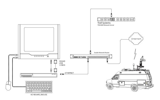
Figure 2–3. Typical VanLink Network Configuration
